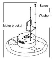
steering motor & steering wheel assembly
