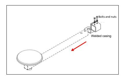
2. Assemble the antenna bracket. Insert the two GNSS antenna assembly into the antenna connector, align the four holes, and fix the suction cup bracket to the antenna assembly with 4 hexagon head bolts M8x50, spring washers 8, 8 flat washers 8 and hexagon nuts M8.
