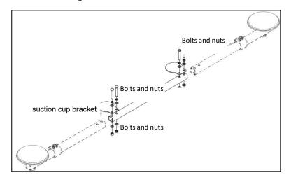
3. Install the antenna bracket assembly on the ceiling of the vehicle. Ensuring the 2 GNSS antennas are symmetrical and perpendicular to the body center of vehilcle by adjusting the position of the casing weldment. After that, tighten 4 hexagon nuts M5 so that the antenna bracket assembly cannot move leftwards and rightwards, and then fix the antenna assembly through the screws on the ceiling.
