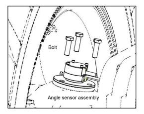
6. Install the fixing bracket. Connect the angle sensor assembly and fixing bracket with 2 hexagon bolts M5x16, hexagon nuts M5, spring washer 5 and plain washer 5, and then fix the fixing bracket with the front axle using 2 hose hoops.
