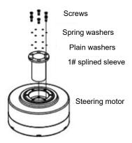
3. Install FJD steering wheel and fix the wheel and motor with 6 hexagon socket screws M5×16, spring washer 5 and plain washer 5.
