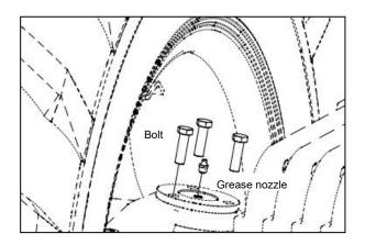
Install the angle sensor assembly. Fix the assembly with bolts removed in step
