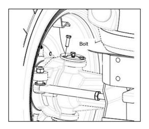
2. Install the attitude sensor assembly on the front axle. Adjust the position of the wiring harness, and then tighten the original bolts to the front axle.
