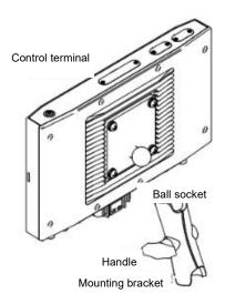
3.Install control terminal installed in step 3 onto the base ball head and rotate it clockwise to ensure that the control terminal is fixed firmly without shaking.
