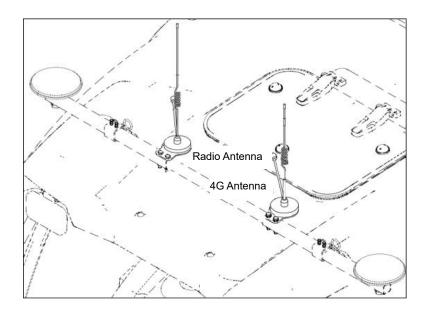
\*The right-hand side of the vehicle forward direction should be GNSS antenna 1, the left side should be GNSS antenna 2. Please follow this instruction to connect the corresponding antenna feeder.
