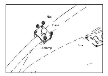
2. Rotate the mounting bracket handle counterclockwise and install the control terminal into the ball socket of the mounting bracket.
