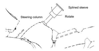
3. Put the 1# splined sleeve into the steering motor, and fix the splined sleeve and steering motor with 6 hexagon socket head cap screws M4×14, 6 spring washers 4 and plain washers 4.
