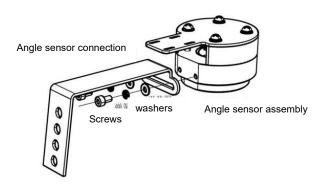
6. Install the angle sensor bracket. Please fix angle sensor assembly and its bracket with 2 cross recessed countersunk head screws M5x8.
