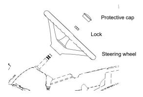
2.Select the splined sleeve according to the spline of the steering column. Install the splined sleeve on the steering column and rotate it leftwards and rightwards until no shaking and clearance is involved.
