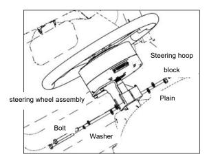
6. Install the original lock nut removed in step 1, and then install dust-proof cap and bonding logo.
