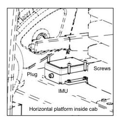
Note: The IMU shall be placed horizontally, with the plug in the direction same as the traveling direction of the vehicle.
