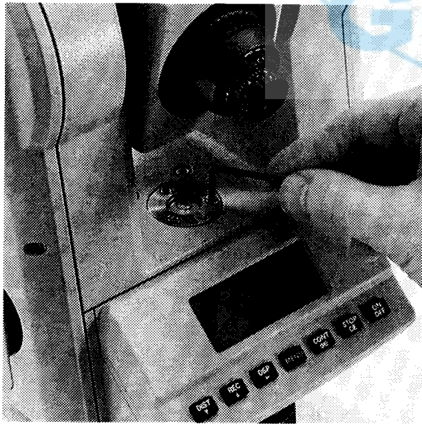
Figure 4: Adjusting the spherical level
