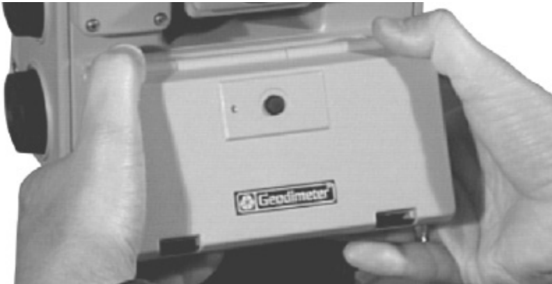
Figure 12.1 How to attach the card memory on an instrument
