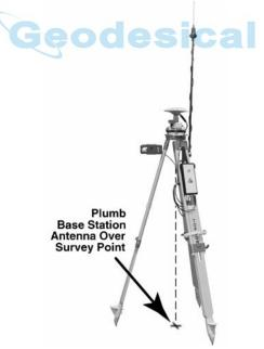
Figure 3-11. Legacy-E with PG-A1 Antenna Base Station Setup
