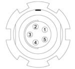
Figure B-3. USB Connector for GGD Options
