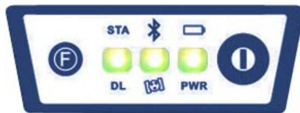
Fig. 2.13 - S9 six lights blinking at the same time
