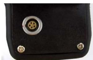
Fig 3.4 - 5-pins interface (for receiver and power supply)
