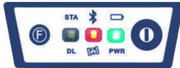
Fig. 2.24 - Bluetooth and external power lights
