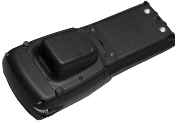
Figure 7.9 Scanner Module Installed In WORKABOUT PRO
