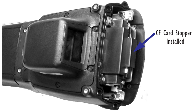
Figure 6.4 CF Stopper Installed
