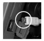
Be sure the direction of USB mini B connector is same as that of the USB port.
