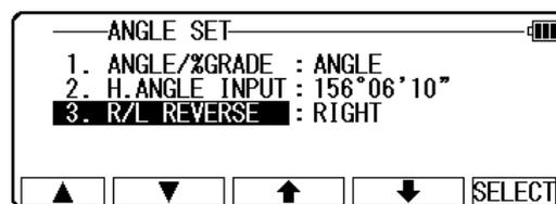
Press [F5] [SELECT] to add a minus sign (-) to the horizontal angle value as a counter clockwise angle.
