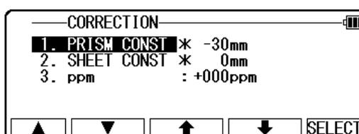
Press [F4] [↓] to move the cursor to “3. ppm” and press the [F5] [SELECT] to enable the temperature to be changed.
