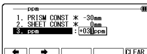
Press the [ENT] key to accept the PPM to 31ppm.
