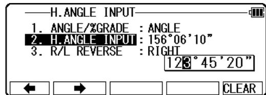
Press the [ENT] key to accept the horizontal angle set to 123° 45' 20" and change the screen.
