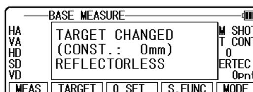
Pressing [F2] [TARGET] changes the target mode.
