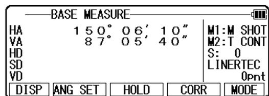
Press [F2] [ANG SET] to display the ANGLE SET screen, then press [F4] [↓] to move the cursor to "2. H.ANGLE INPUT".
