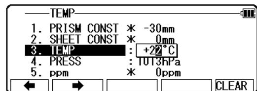
Press the [ENT] key to accept the temperature to +22°C.
