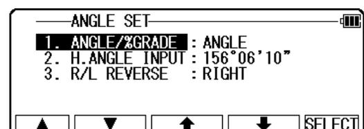
Press [F5] [SELECT] to open the horizontal angle input window.
