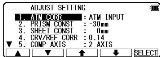
Press [F5] [SELECT] to open the screen for selecting the atmospheric correction.
