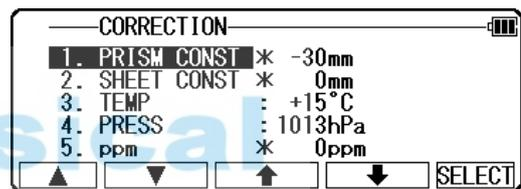
Press [F4] [↵] to move the cursor to “3.TEMP” and press the [F5] [SELECT] to enable the temperature to be changed.
