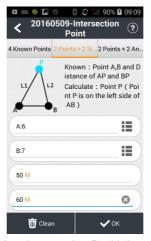
**Points + 2 Angles**: Calculate intersection P with known points A and B and the inner angle of PAB. Click **OK** to calculate. Input a name, and click **OK** to save.
