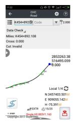
**Free Slope**: When meet slope with same type, you can select free slope to avoid duplication input.
