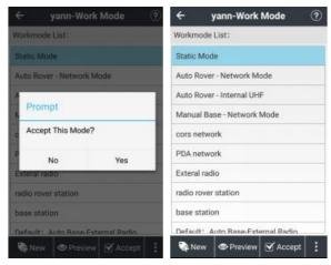
**Use PPK function**: When you finish setting base station (Static mode), it is necessary to set other receiver as rover station which uses PPK function. You can click to set **PPK Obs Time Config** based on satellite numbers. Afterwards, click OK, the PPK function can operate and the time will show in interface which based on the numbers of searching satellites. Beside, we provide auto complete to conveniently save static data without watching the static recording internal time.
