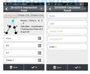
**Points + 2 Sides**: Select points A and B from point management. Enter the length of line AP and line B. Click **OK** to calculate. Input a name, and click **OK**
