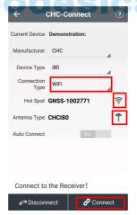
**Demonstration**: Enter Demo mode, and then users can use or test all the functions of this software. Meanwhile, the function can simulate position by inputting coordinate.
