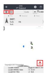
Arrow: Give direction to target point in real time.
