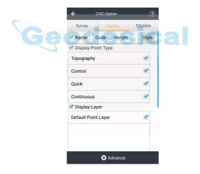
Name/Code/Height: Select to display on Map interface, users can select one item or multi-item. For example, if selecting Name and Code, users will see point name and code on Map interface after measurement.
