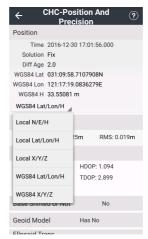
**Precision**: Users can view horizontal precision, vertical precision and RMS.
