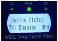
On hot days, it is possible that the radio power setting is higher than the enabled value. Power will also be reduced if
