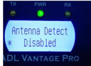
There is a chance that a good antenna will be detected as bad, which will result in inadvertent lower output power and reduced rover range. So if you know your antenna and cable are in good condition leave 'Antenna Detect' set to 'Disabled' to insure continuous high output power.
