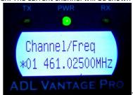
The Base and Rover frequencies should match this setting. Note that the channel number may be different, but the frequencies must match.
