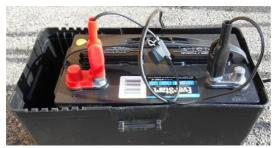
Figure 16 Alligator-clip connections won't support full output power!
