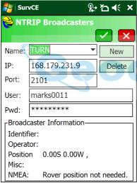
Enter the correct service Name, IP Address, Port, User Name and Password for your network. (The example above shows 'The Utah Reference Network' or TURN. Both the 'User Name' and Password are case sensitive and must match your network credentials exactly. Double check the settings, then click on the Green Checkmark.
