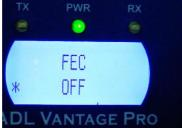
Turning FEC ON lengthens each data packet.
