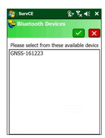
Highlight the correct receiver (the number is the serial number of the device, if you have your Base AND Rover powered up, make sure you are connecting to the Rover!)
