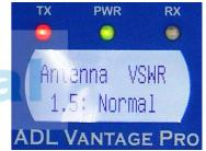
Values higher than 8:1 result in a 'no antenna connected message.'
