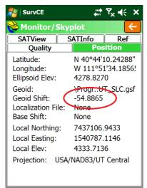
Notice that the GEOID Shift is negative. It is subtracted from the Ellipsoid elevation and causes the Local (orthometric) height to be higher than the ellipsoid. (This is true for most of the planet.)
