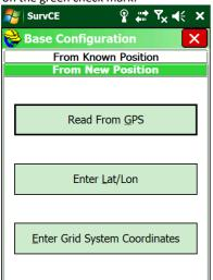
If you don't know the position of the base, click on 'Read From GPS'. If you have a geographic coordinate (Latitude / Longitude), then you can hand enter the position using either 'Enter Lat/Lon'. Use 'Enter Grid System Coordinates' if you know the Grid Coordinates for the base position or if they are an existing point in your job. If you have previously setup on the point, you can use the 'From Known Position' tab.
