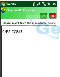
Your Base will have its Serial Number on a sticker on the bottom of the head. Click the correct device to select it, then click on the green check mark.
