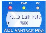
NOTE: 50% of all RTK Radio Problems are due to incorrect Radio Link and Serial Baud Rate settings.
