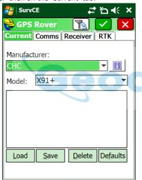
Select Manufacturer 'CHC' and Model 'X91+' or 'X900+' (to match your receiver.) Note that there is a 'X91+' and a 'X91' (with no '+'); select the correct model.
