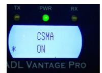
When CSMA is turned ON, the radio will listen for other data or voice users on the programmed frequency, the radio will wait until other users stop broadcasting before transmitting. FCC rules require CSMA to be ON for operation in the United States.
