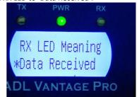
The RX LED will blink only when complete, valid transmissions are received from the Base.
