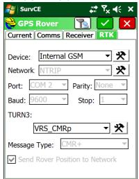
Click the green check mark again. The rover will connect to the correction source, the green 'radio' led on the receiver will start to flash.
