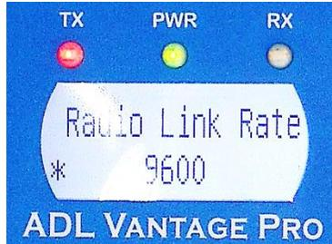
NOTE: 50% of all RTK Radio Problems are due to incorrect Radio Link and Serial Baud Rate settings.
