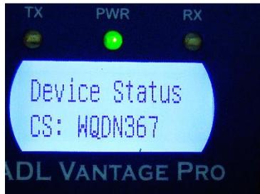
A valid FCC license is required for operation in the United States and the FCC assigned ID must be transmitted by continuous wave (CW) Morse Code every 15-minutes.
