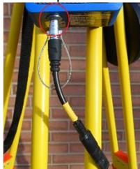
4. The radio will turn on when power is applied. **IMPORTANT:** Before you remove power from the radio, ALWAYS turn the radio off with the power switch. Push and hold the Power ON/OFF button for five seconds, then wait for the radio to power down:
