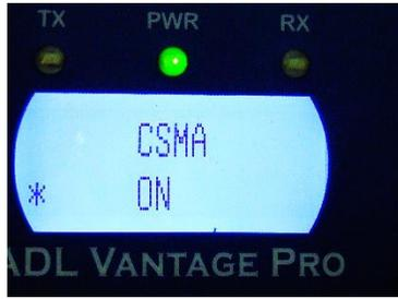
When CSMA is turned ON, the radio will listen for other data or voice users on the programmed frequency, the radio will wait until other users stop broadcasting before transmitting. FCC rules require CSMA to be ON for operation in the United States.
