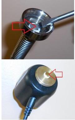
2. Connect the UHF Radio antenna to the radio mast, connect to the antenna port on the ADL Vantage Pro.
