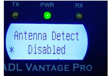
There is a chance that a good antenna will be detected as bad, which will result in inadvertent lower output power and reduced roover range. So if you know your antenna and cable are in good condition leave 'Antenna Detect' set to 'Disabled' to insure continuous high output power.
