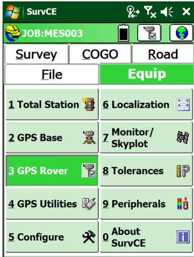
15. You can check the receiver status using “Equip: 7 Monitor Skyplot”:
