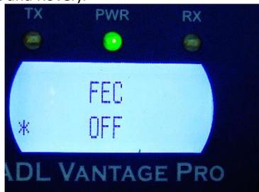
Turning FEC ON lengthens each data packet.
