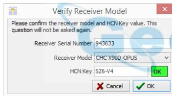
Use the drop down 'Receiver Model' to change the receiver type. If the HCN Key has been lost, it is written on a white sticker inside the battery compartment. You cannot edit the 'Receiver Serial Number'.
