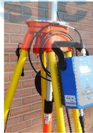
Prism pole through tripod head
