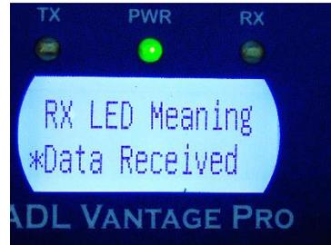
The RX LED will blink only when complete, valid transmissions are received from the Base.
