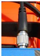
DO NOT plug power into the ADL radio until the UHF antenna has been connected and placed on the mast.
