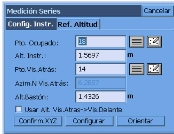
The screenshot shows the 'Medición Series' dialog box with the 'Config. Instr.' tab selected. The 'Ref. Altitud' sub-tab is also active. The fields are: Pto. Ocupado: 18; Alt. Instr.: 1.5697 m; Pto. Vis. Atrás: 14; Azim. N Vis. Atrás: 6.2857; Alt. Bastón: 1.4326 m. There is a checkbox for 'Usar Alt. Vis. Atrás->Vis. Delante' which is unchecked. At the bottom are buttons for 'Confirm. XYZ', 'Configurar', and 'Orientar'.
