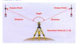
TKS-202 Total Station can determine the azimuth and coordinates with certain known points. This function is especially useful if the coordinates of the specific instrument station is unknown. Elevated station from two known reference points can also be calculated, with each deviation of multiple reference points being displayed.
