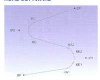
The on-board ROAD software satisfy your massive application measurement by automatically calculating complicated spiral curve and a long distance route by defining only the required points (start point, terminal point or curvilinear point) according to your needs.
