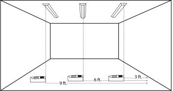
Stake out specific distances or use in tracking mode for continuous measurement
