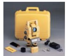
GTS-820A ..... Battery BT-56Q...... Battery charger BC-27BR (120V) or BC-27CR (230V) ..... Tool kit with case..... Plastic carrying case.....1 each Silicon cloth ..... Plastic rain cover ..... Plumb bob set ..... ....1 each Lens cap ...... Instruction manual ......
