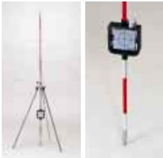
A 50 x 50 mm, 360° rotating sheet target, the RT50P can be connected to narrow pin poles.
