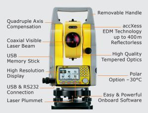
The GeoMax Zoom20 Pro Manual total station includes an environmentally protected USB port that allows fast, simple and reliable data transfer between the instrument and your PC, even to other total stations.
