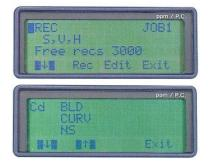
Sophisticated Application Software Missing Line Measurement (MLM) •The SET5F measures horizontal distance, slope distance, height difference, and slope in percent (%) between two prisms, all at the touch of a key.
